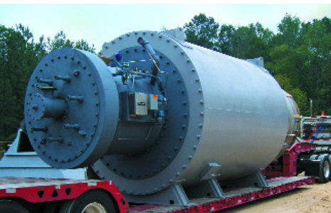
A 115 MM Btu HGG being transported to site.
