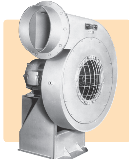
2400-G Blower filter or SW inlet adapter can be furnished in place of guard. Discharge position #3 is shown. It can be changed in the field to any other position shown on the back.
