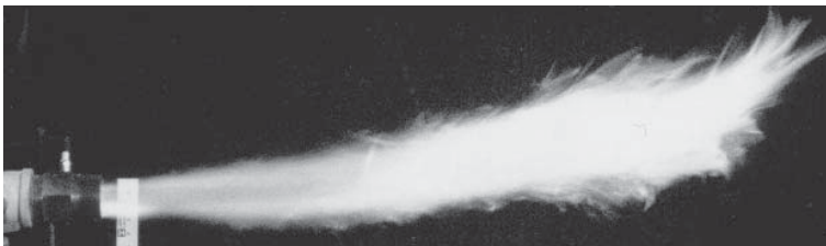
2 1/2" 4020-HP Nozzle-Mix Pilot Tip 100% excess fuel 8 psi air pressure
